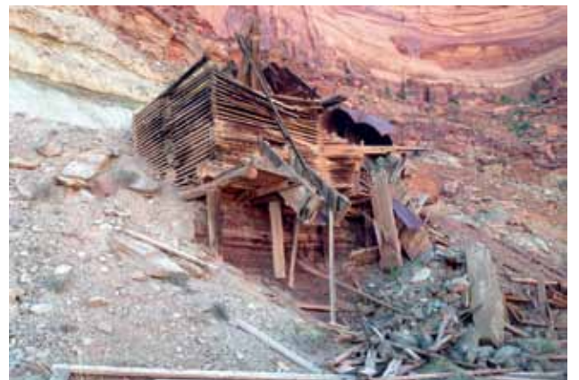
An uranium ore-loading bin in the Chinle Formation used during the boom days when many small mines were active near Moab
