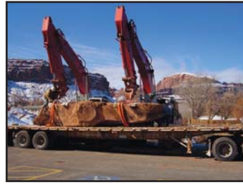
An estimated 30 tons, King World rock required precision movement by heavy-equipment operators to avoid damage.
